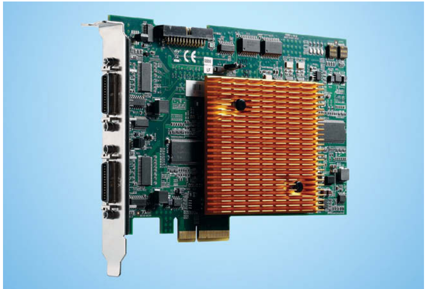
ADLink’s PCIe-CPL64 frame grabber supports Power over Camera Link and a two-channel Camera Link base configuration and performs onboard preprocessing. Courtesy of ADLink Technologies.
